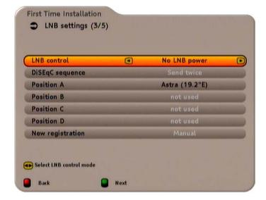
Press the 🔊 buttons to switch to the "Position A". Press the 🕟 button to open the sub-menu. You can select a satellite and make the related settings here. Press the 🖣 (green) button. If you change the default setting (in this example "ASTRA 19.2°E"), a prompt "Save LNB settings?" will be displayed. Select "Yes" or "No" using the 🕦 buttons and accept your selection using the 🕩 button.
